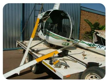
From what I can piece together, from blurred memory and having looked at the photographs of the wreck, is that flaring the tail through the trees to bleed off our speed had caused us to lose our tail rotor. With the loss of torque, RFV smashed left-side into the trees, putting Carlos in the direct path of the highest impact, throwing him out, and then underneath the helicopter while still suspended by his monkey harness.
